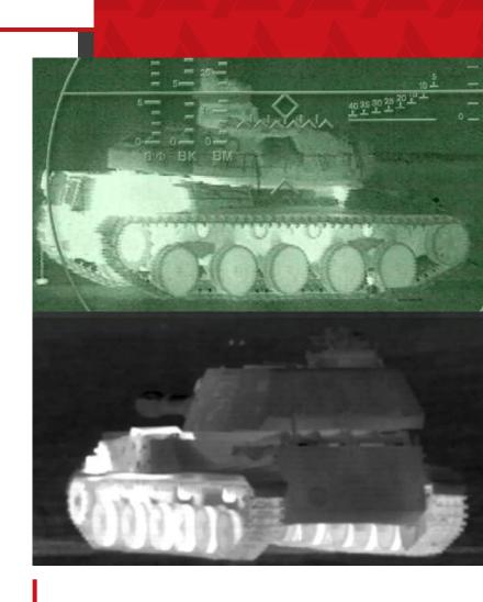
Heating of the power plant strongly unmasks armored vehicles in the thermal range
