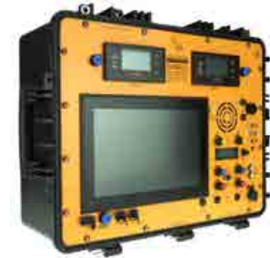
ALPHEUS-C1 | Portable diver radio, video recorder and depth monitor
